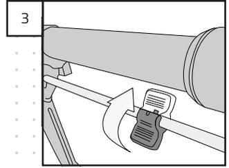
Use the **Tightener** to turn the **Spring Pin** clockwise until the **Left Rod** is completely firm and the **Pin** is in upright position.
