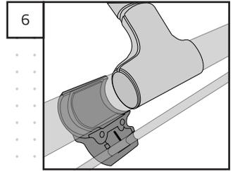
Place **Collar S** behind the drone's arm and the **Left Rod**. Make sure the **Spring Pin** is placed in the middle of the **Collar**.
