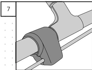
Align the upper parts of **Collar B** and **Collar S**. Snap them into place, ensuring all parts are completely secured and enclosed.
