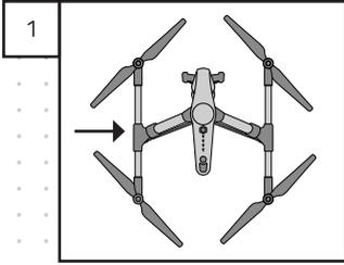
Start mounting the left kit, by facing the left side of the drone. The mounting procedures have to be made in **landing mode**.
