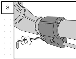
Tighten both screws with the **Hex Key** to secure the **Collars**. Be careful not to deform the plastic components.
