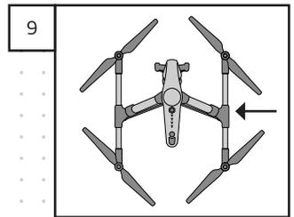
**RIGHT ROD:** Please note that the **Right Rod** follows the same procedure as the left, but the rod needs to be screwed **counter clockwise**.
