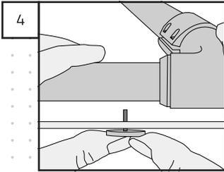
Use a coin or any other sturdy tool to push the **Spring Pin** up until it sticks out from above the **Rod** only.
