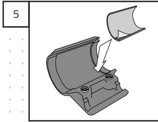
Place the adhesive strips on the inside of **Collar B** and **Collar S**.
