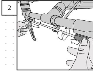
First place **Clamp A** around the landing gear and insert the **Left Rod** into the hole. Repeat the procedure on the other side placing **Clamp B** and screwing the **Left Rod** clockwise.
